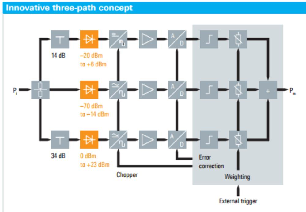
**Figure 1-1: Multipath sensors offer the widest measurement range and fastest speeds by utilizing separate diode paths for different power ranges.**
