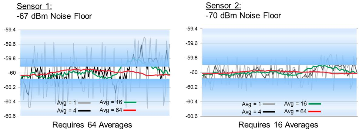
**Figure 2-4:** In this example, two sensors with similar speeds and uncertainty, but one having a lower noise floor, gets the same results four times faster.
