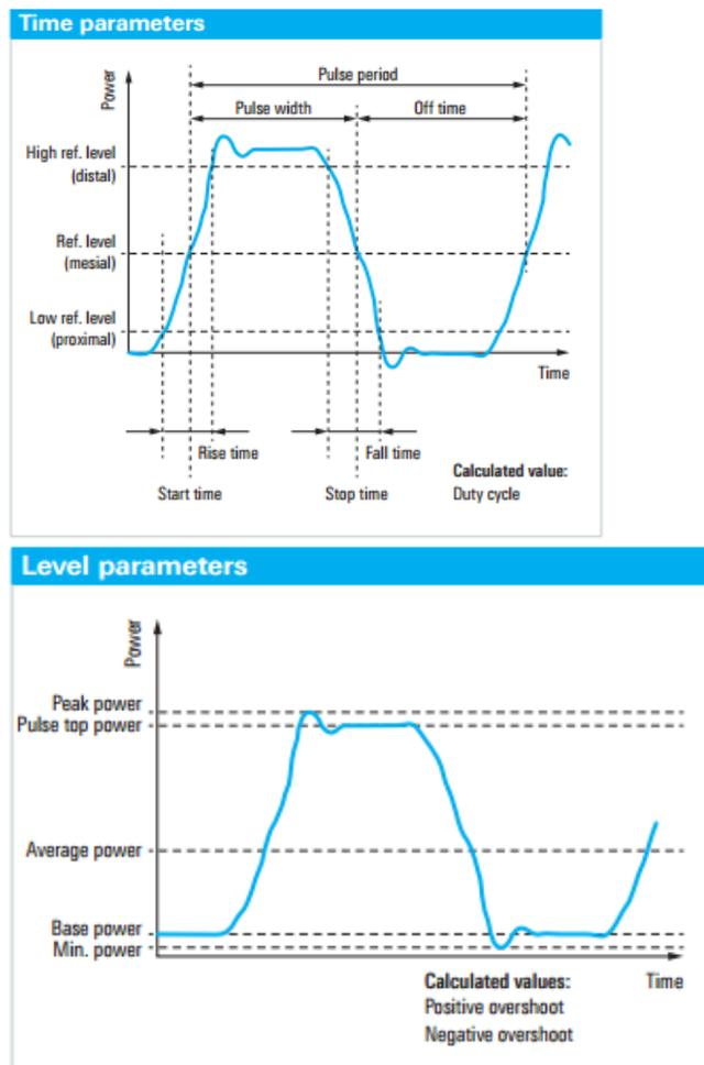
Figure 1-3: Wideband sensors offer more measurement types, such as envelope statistics, pulse analysis, and time analysis.
