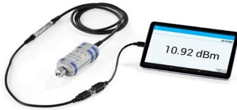
**Figure 3-1: USB based power sensors are the most popular today due to their flexible control interface and portability.**
