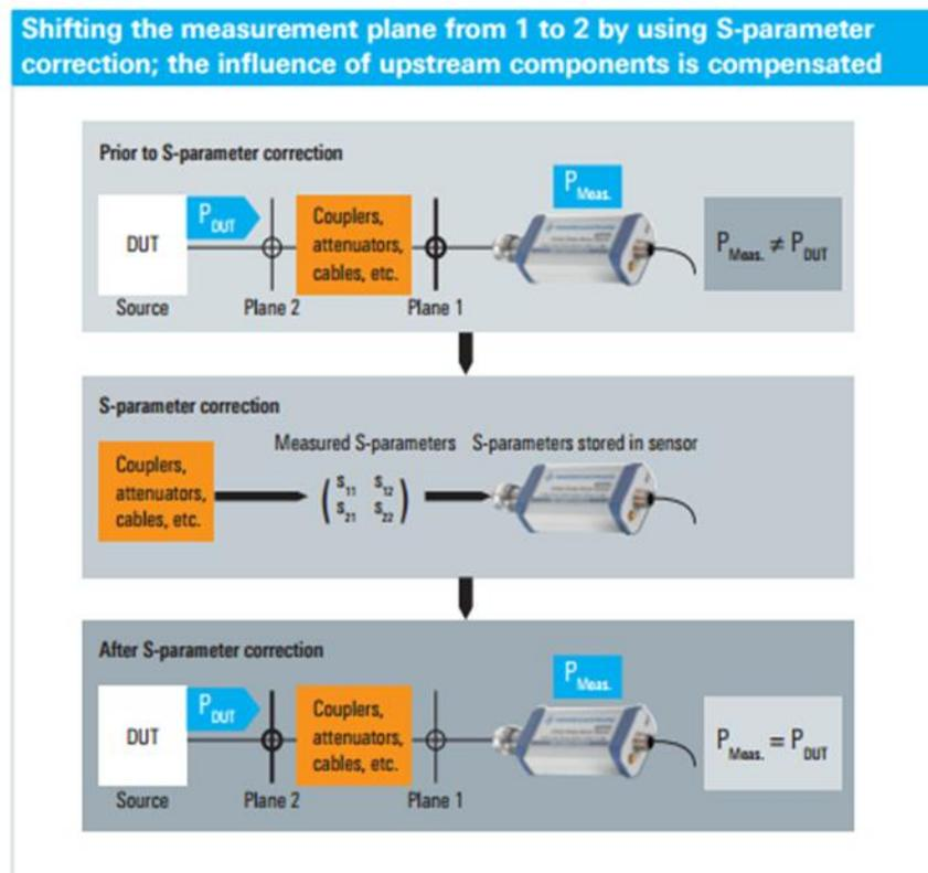
Figure 2-3: Use S-parameters to compensate for external components and improve uncertainty.
