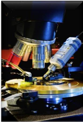
**Figure 1-4: Thermoelectric power sensors are especially used in calibration labs and demanding applications that require high performance reference measurements.**
