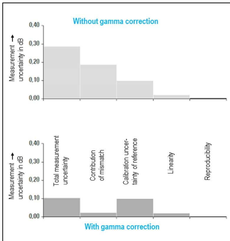
Figure 2-2: Gamma Corrections may be used to limit the impact of mismatch on the overall test setup uncertainty.
