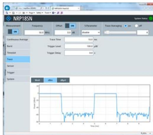
**Figure 3-2:** LAN sensors are ideal for ATE systems or remote monitoring site and offer a built in web server that allows for real-time monitoring from multiple locations.
